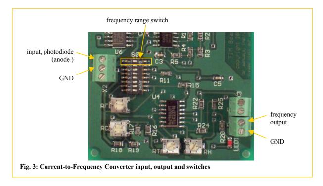
If there appears no pulse signal on the output the polarity of the photodiode may be wrong. Also check that your equipment is able of recognising pulses as short as 1 µs. Especially with older analog oscilloscopes and under artificial illumination it can be tricky to trigger these pulses because the output frequency may vary with the double of the mains frequency.
